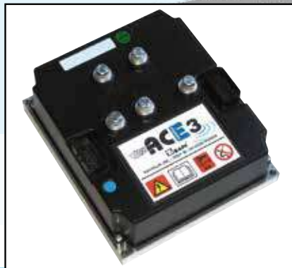
PUMP CONTROLLER: ZAPI ACE-3
